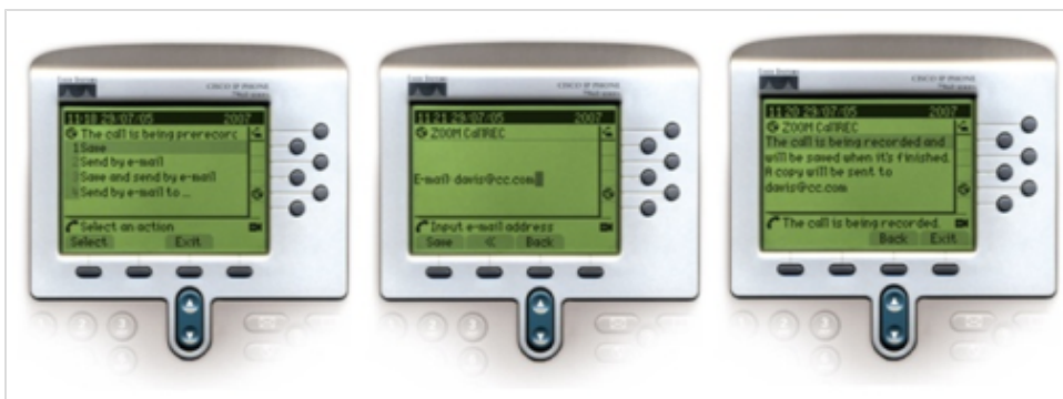
Figure 21: Call Recording User Interface on an IP Phone
